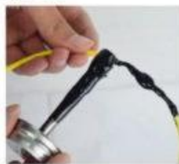
2. Apply liquid tape to wire
